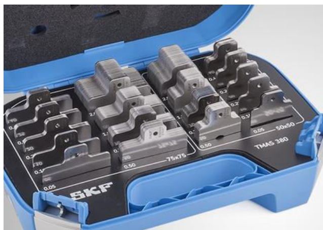
SKF kalibrisani podmetači (shims)
